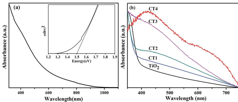
Fig. 5 UV-vis DRS spectra for: (a) as-synthesized CZTS nanoparticles, with the inset showing the determined band gap value of 1.5 eV; (b) CZTS–TiO<sub>2</sub> samples CT1, CT2, CT3 and CT4, which stand for, respectively, 1.9, 3.8, 5.7 and 7.6 mg of CZTS in 0.1 mL of TiCl<sub>4</sub>.
