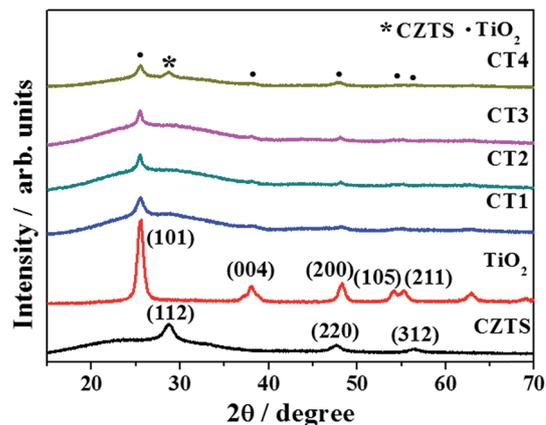
Fig. 4 XRD pattern for as-synthesized CZTS, TiO<sub>2</sub> and hybrid CZTS-TiO<sub>2</sub> samples (CT1, CT2, CT3 and CT4 stands for 1.9, 3.8, 5.7 and 7.6 mg of CZTS in 0.1 mL of TiCl<sub>4</sub> respectively).
