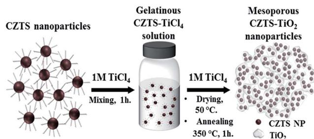
Fig. 1 Schematic showing the experimental strategy for synthesis of hybrid mesoporous CZTS–TiO<sub>2</sub> photocatalyst.
