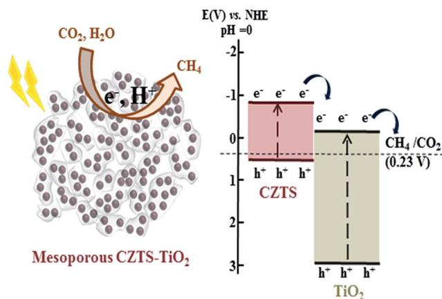
Fig. 8 Schematic illustration for photocatalytic CO<sub>2</sub> conversion into methane by hybrid CZTS–TiO<sub>2</sub> samples with proposed energy level diagram.
