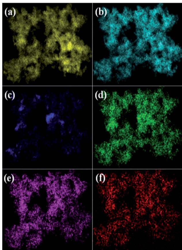
Fig. 3 EDX-STEM elemental mapping image of CT4 sample showing composition of: (a) titanium, (b) oxygen, (c) copper, (d) zinc, (e) tin, and (f) sulphur.
