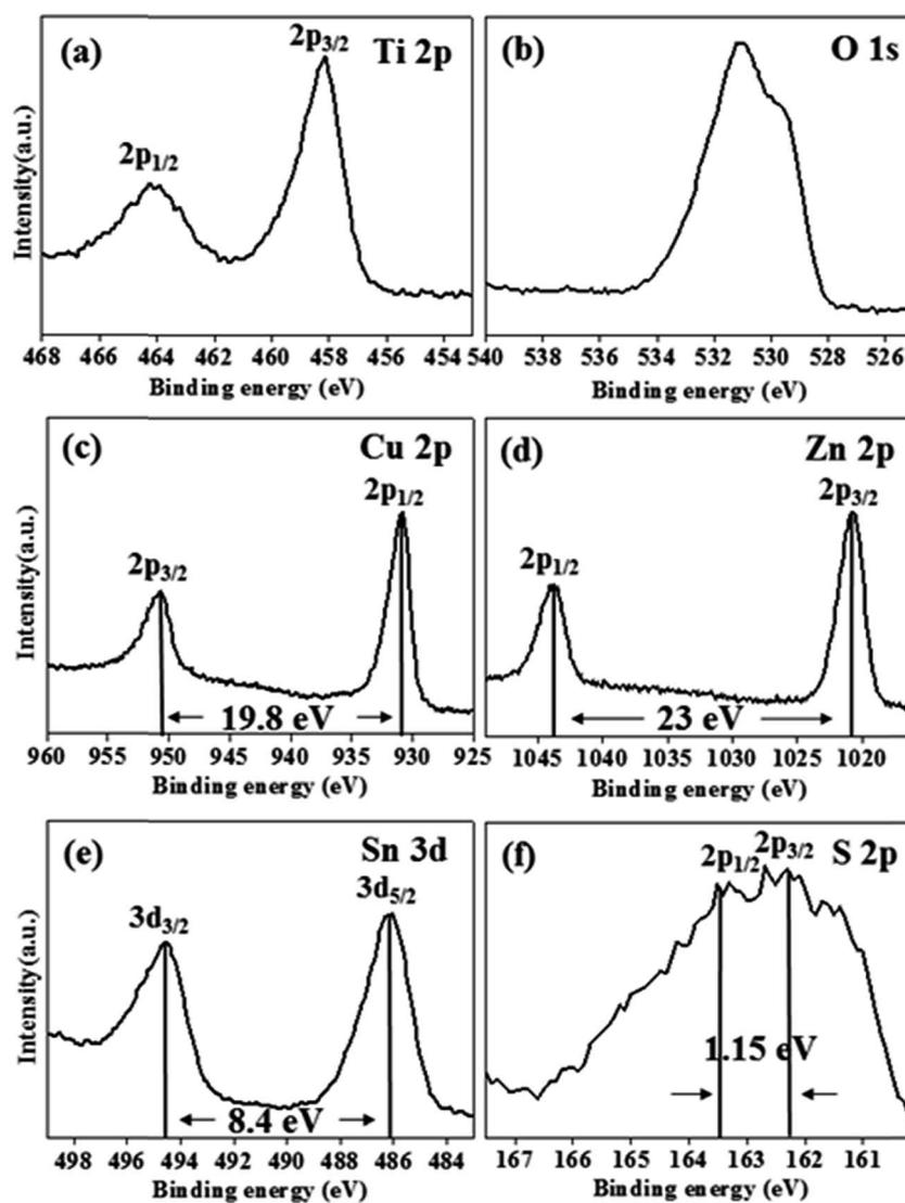
Fig. 6 X-ray photoelectron spectroscopy (XPS) of CT4 sample with regions of: (a) titanium, (b) oxygen, (c) copper, (d) zinc, (e) tin and (f) sulphur.
