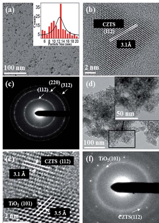
Fig. 2 TEM, HRTEM and SAED patterns of: (a–c) as synthesized CZTS nanoparticles; and (d–f) CZTS– $\text{TiO}_2$  sample CT4.
